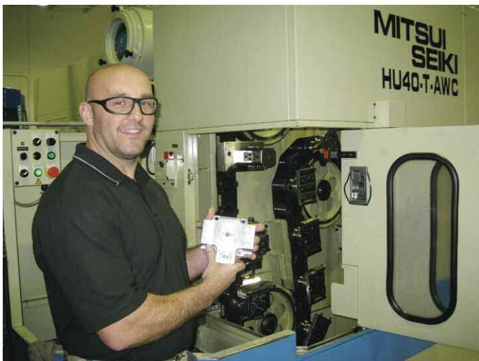
Dominic Teague, Magnus Precision Manufacturing, shows one of the complex parts machined 'lights out' on the Mitsui Seiki HU40-T-AWC 5-axis machining center.
